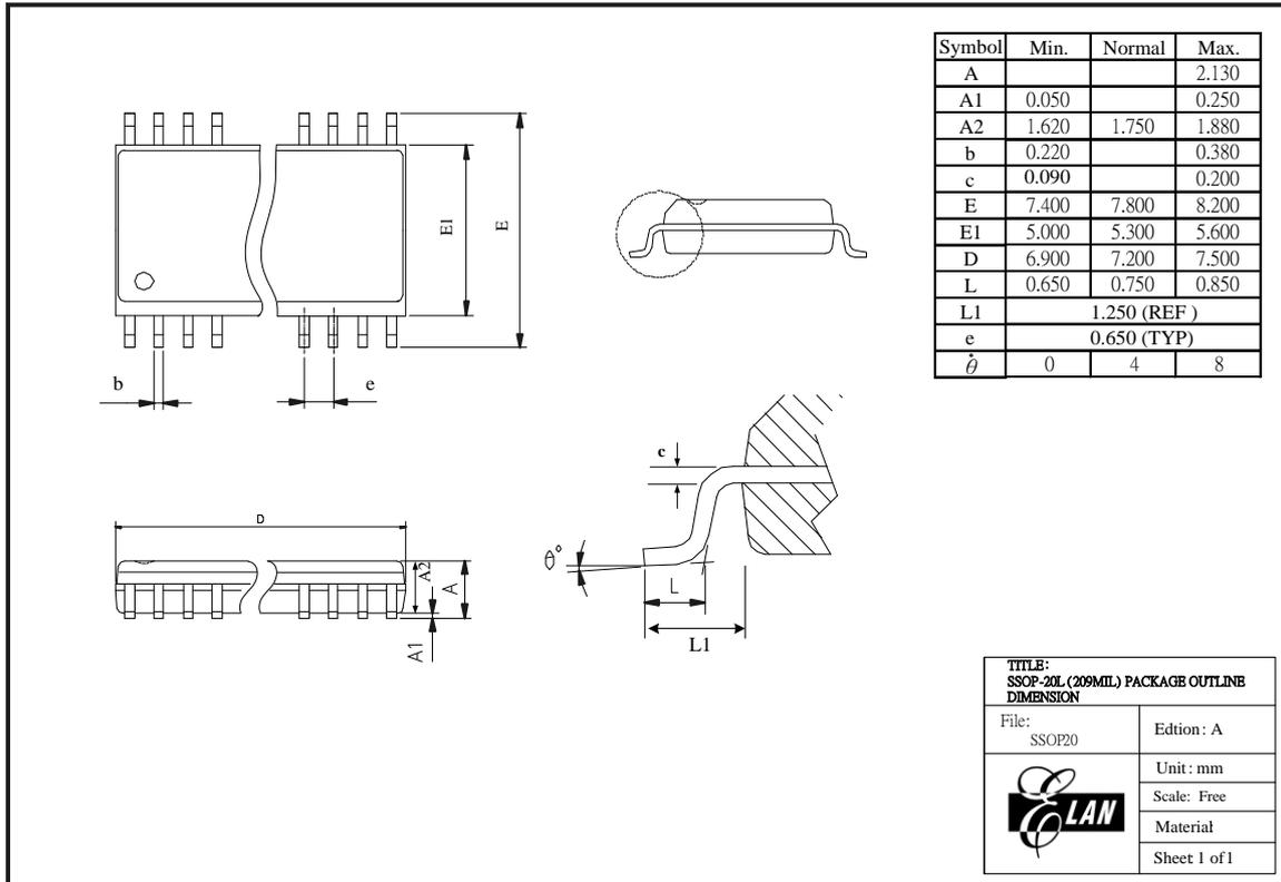
Figure C-8 EM78P259N 20-pin SSOP Package Type
