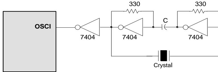
Figure 6-18 Serial Mode Crystal/Resonator Circuit Diagram
