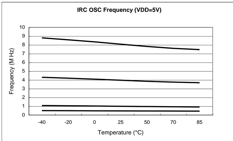
Figure 8-2 Internal RC OSC Frequency vs. Temperature, VDD=5V
