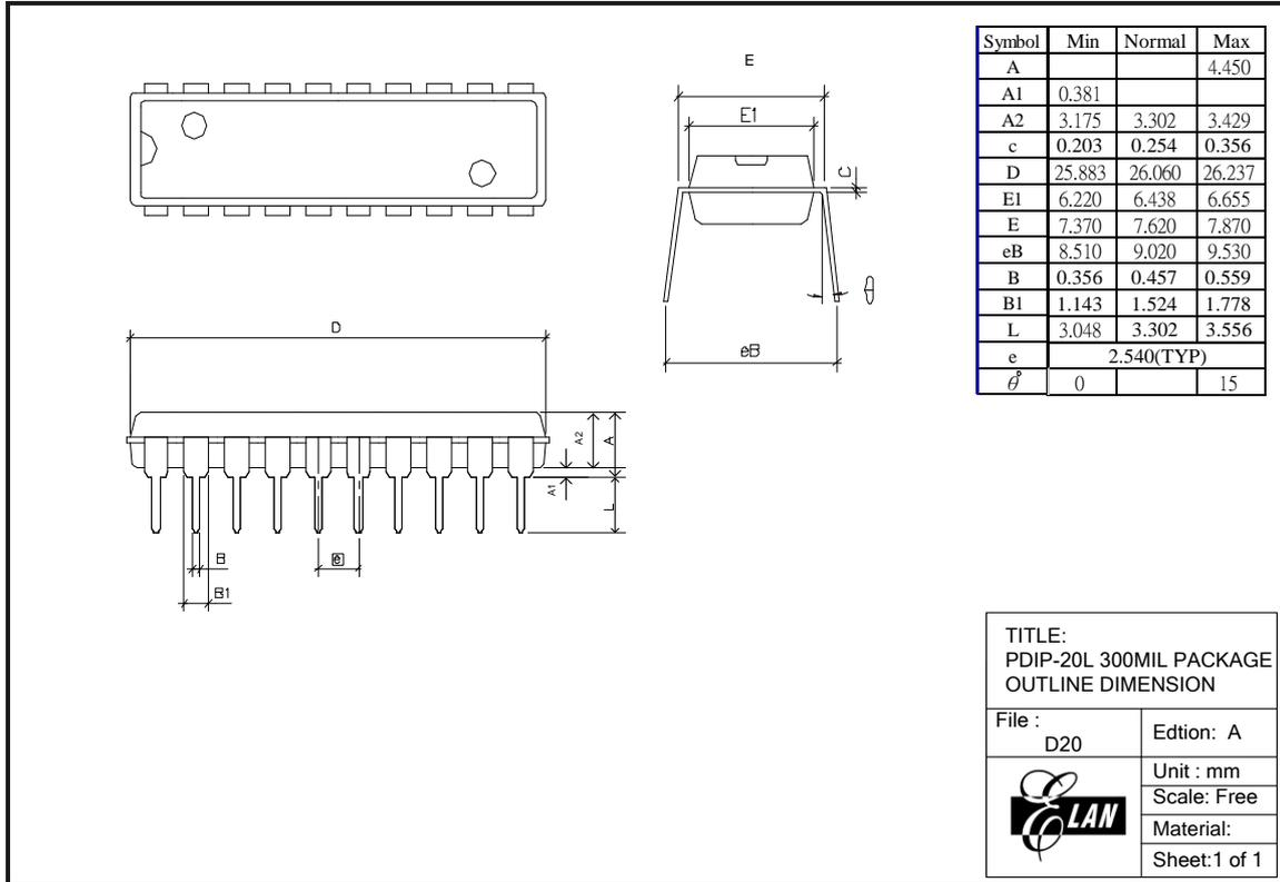
Figure C-6 EM78P259N 20-pin PDIP Package Type
