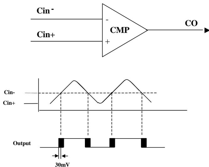
Figure 6-14 Comparator Operating Mode
