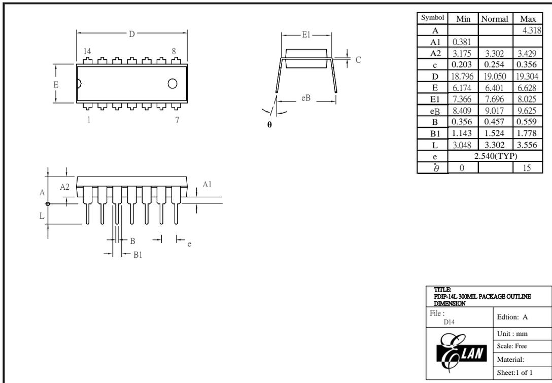
Figure C-1 EM78P259N 14-pin PDIP Package Type
