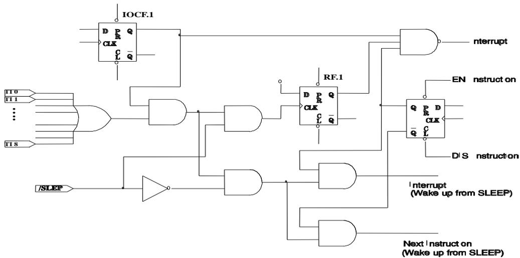
Figure 6-6 Port 5 Block Diagram with Input Change Interrupt/Wake-up
