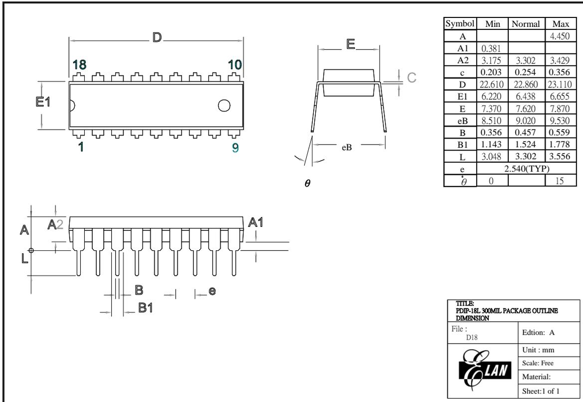
Figure C-4 EM78P259N 18-pin PDIP Package Type
