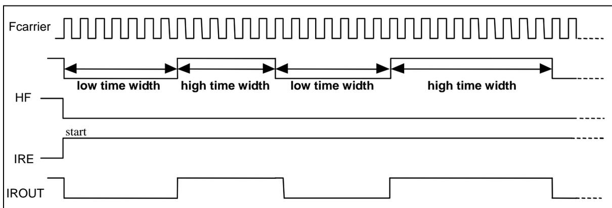
Figure 6-12b LGP=0, HF=0, IROUT Pin Output Waveform
