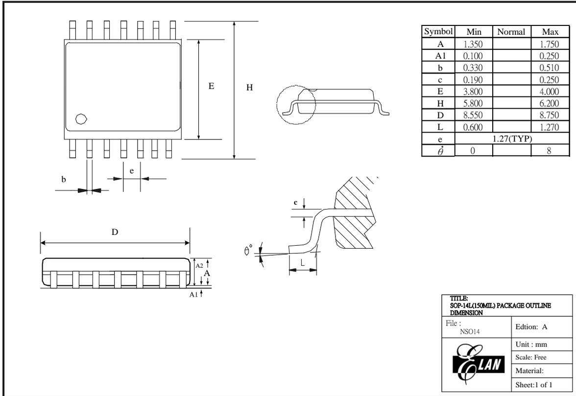
Figure C-2 EM78P259N 14-pin SOP Package Type
