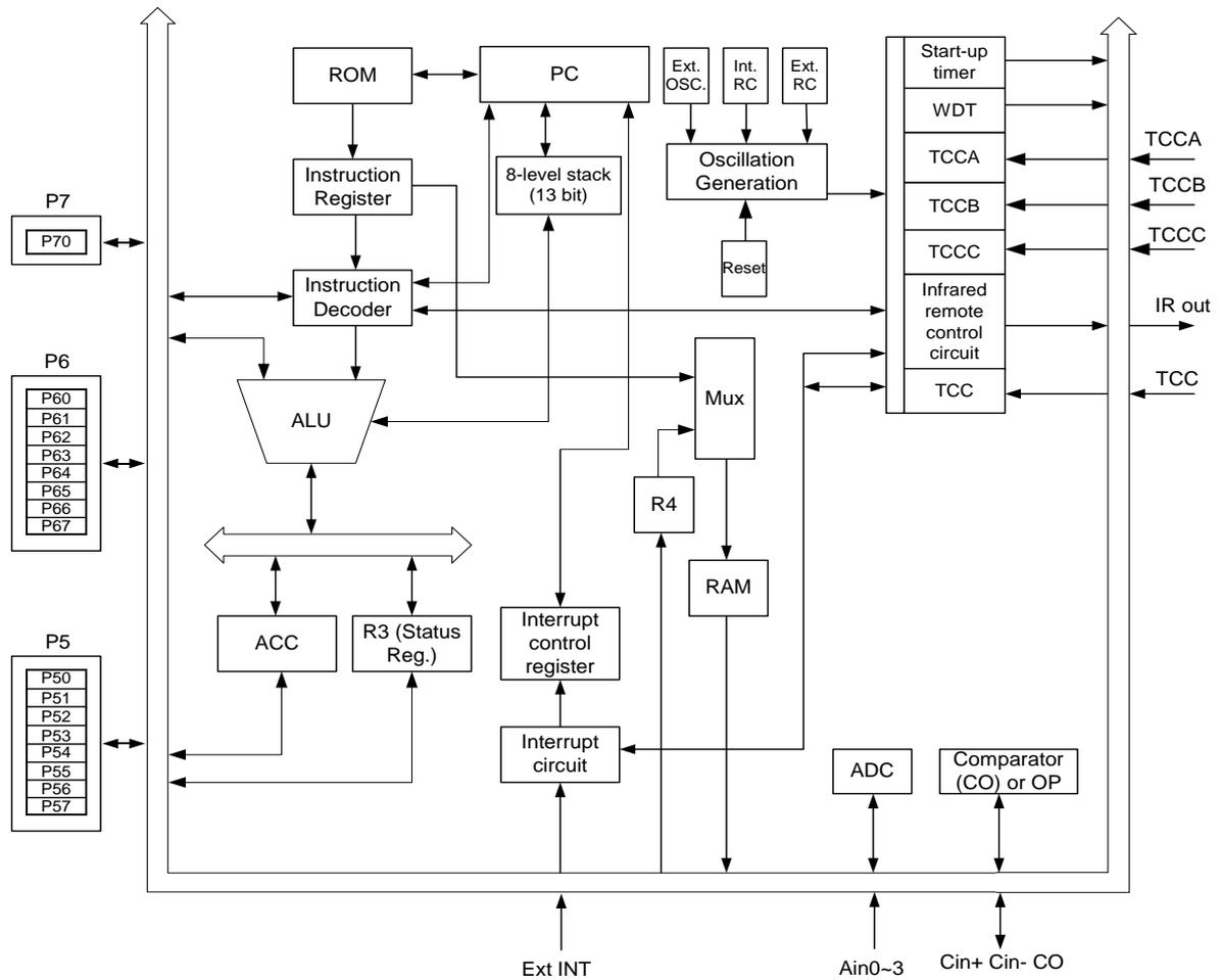
Figure 5 EM78P259N Functional Block Diagram
