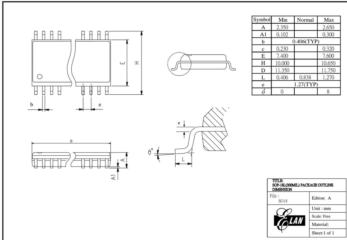
Figure C-5 EM78P259N 18-pin SOP Package Type
