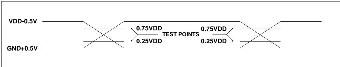
AC Testing : Input is driven at VDD-0.5V for logic "1", and GND+0.5V for logic "0". Timing measurements are made at 0.75VDD for logic "1", and 0.25VDD for logic "0".
