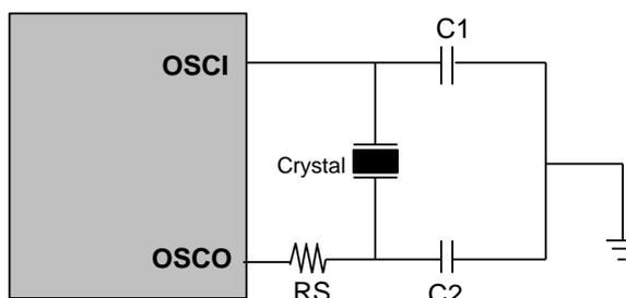
Figure 6-17 Crystal/Resonator Circuit
