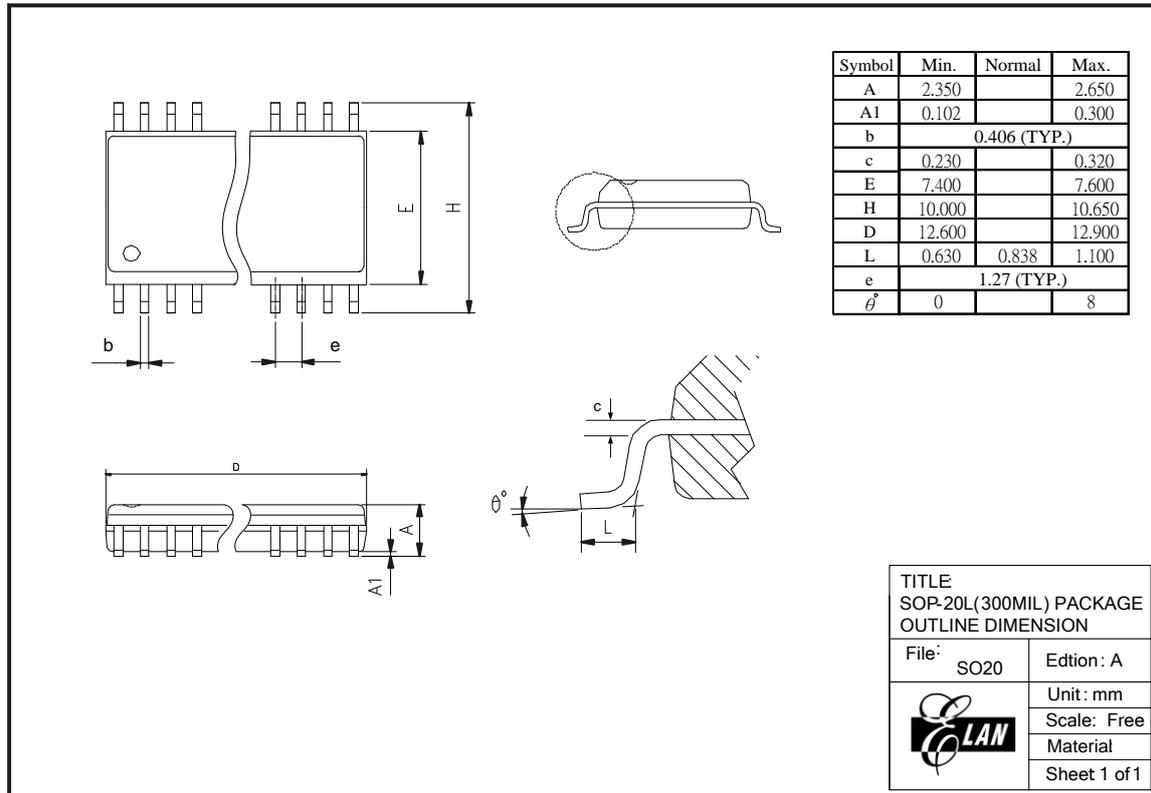
Figure C-7 EM78P259N 20-pin SOP Package Type
