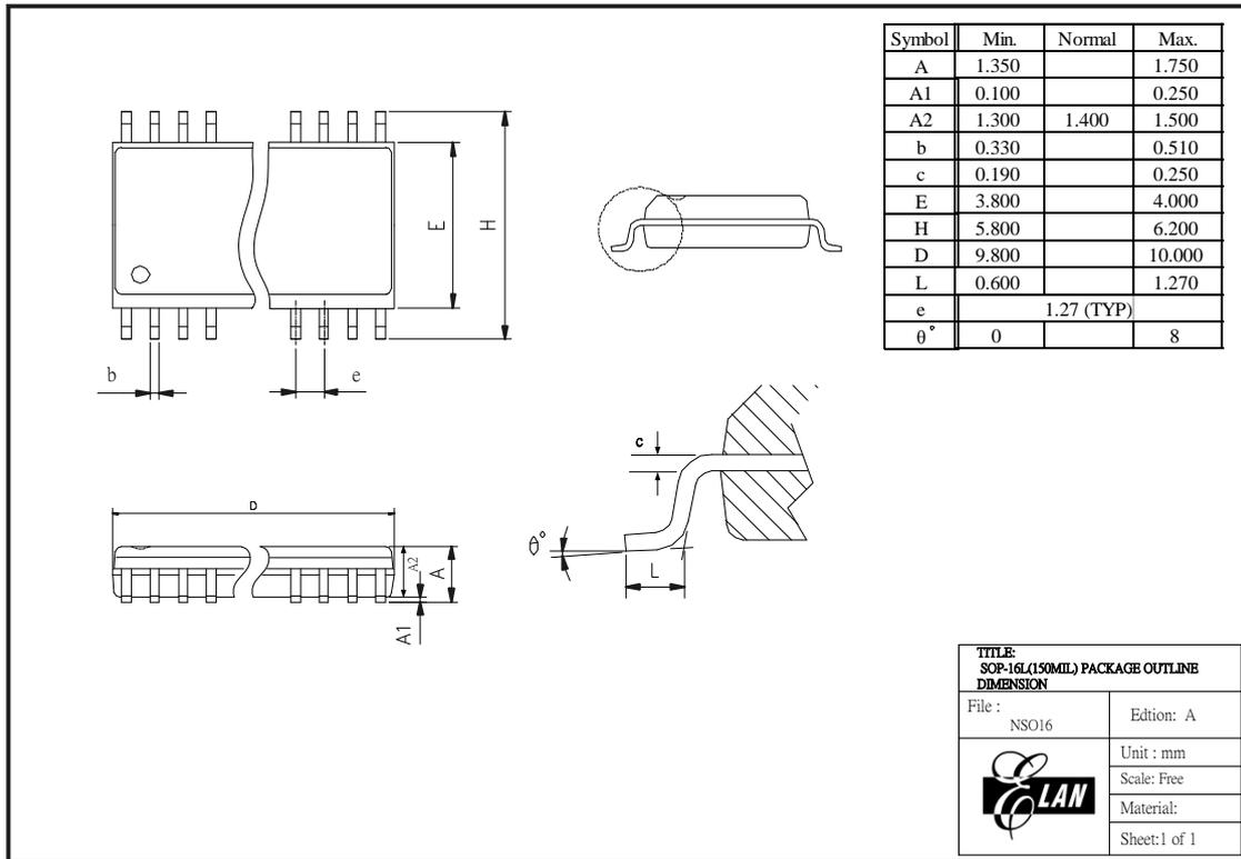
Figure C-3 EM78P259N 16-pin SOP Package Type
