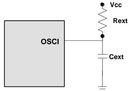
Figure 6-20 External RC Oscillator Mode Circuit
