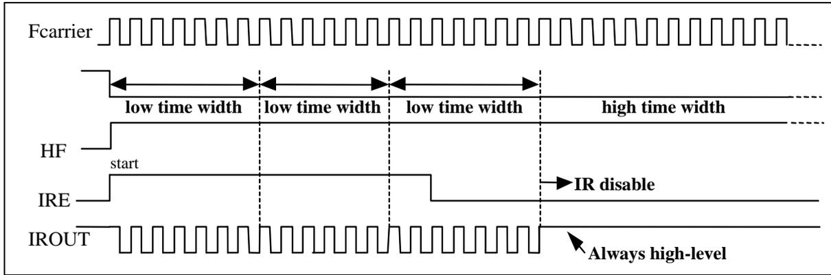
Figure 6-12e LGP=1 and HF=1, IROUT Pin Output Waveform
