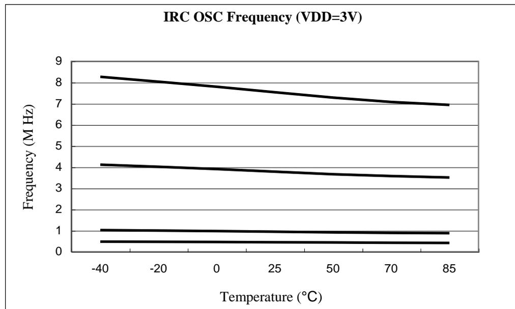
Figure 8-1 Internal RC OSC Frequency vs. Temperature, VDD=3V
