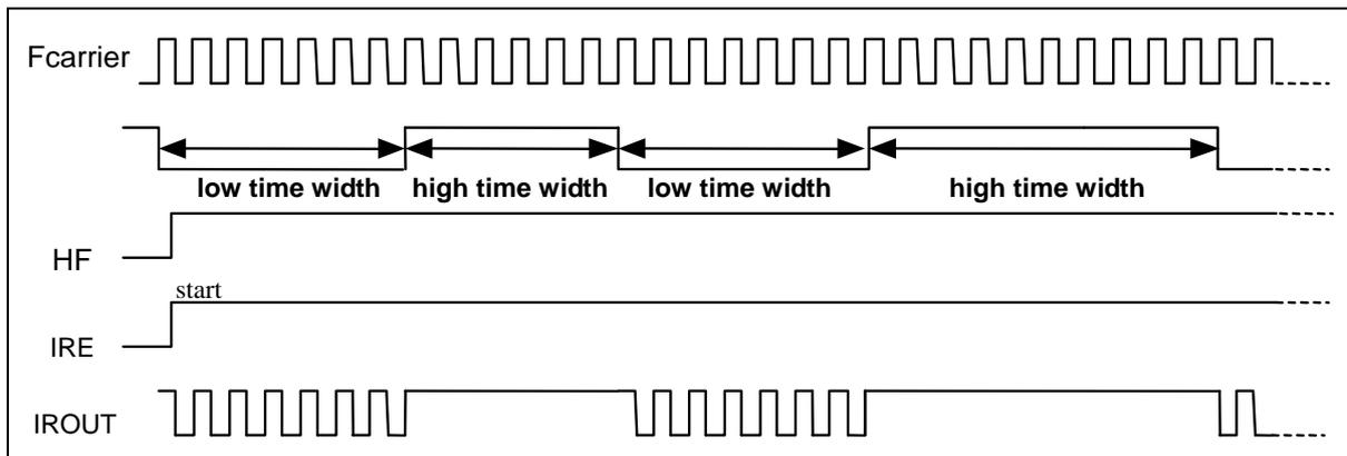
Figure 6-12a LGP=0, HF=1, IROUT Pin Output Waveform
