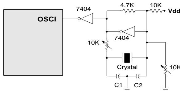
Figure 6-19 Parallel Mode Crystal/Resonator Circuit Diagram
